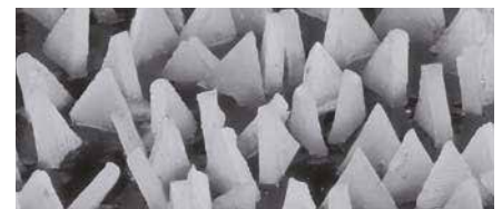
The VICTO GRAIN abrasive grain is optimally aligned
